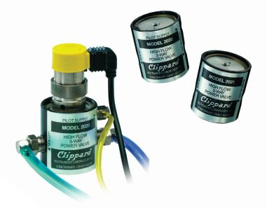
These pressure piloted valves are designed to be piloted by a manifold mount Clippard EV valve (not included). Output from the valve actuates the booster to produce outputs up to 620 l/min at 100 psig (7 bar). Combines low wattage, long life, and cool running of the EV valve with quick response and high flow. Available internally or externally piloted.
